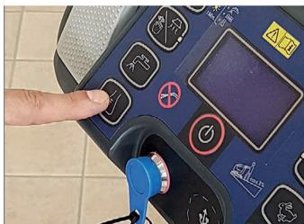
12. Machine with Ecoflex, always end the daily work with turning off the detergent 2 minutes before finishing by pressing the detergent button. To rinse out detergent from the system and brush before handling and cleaning.
