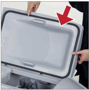
4 Check the lid gasket is in good and working condition and sealing when lid is closed.
