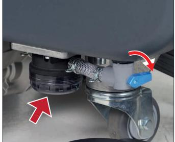
15. Clean the filter: A) Close the solution valve under the machine. B) Remove the transparent cover and the gasket, then remove and clean the filter inside. C) Reassemble the filter.
