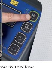
6. Place the user key in the key reader, then start the machine by pressing the One-Touch button. To engage the brush, slightly press the drive paddle and then release it.
