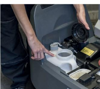
tergent suitable for cleaning machines (highly concentrated and low foaming detergent).
