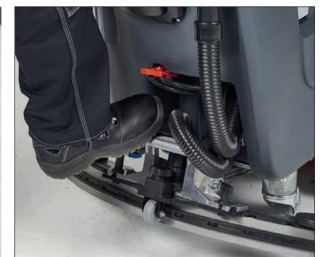
7. Lower the squeegee with the pedal. 8. Push forward the drive paddle to
