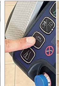
9. To change the solution flow level push the solution button and change flow level according to the cleaning performance and application.
