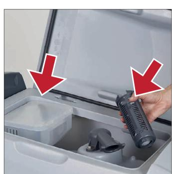
2 Open the recovery tank and check 3 Check if squeegee blades are the debris tray and float are clean and working.
