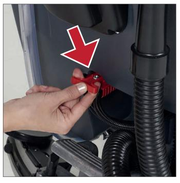
Check if the power cable is correctly connected.
