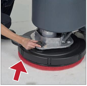
1 To adjust machine direction turn front knob until machine is working straight.
