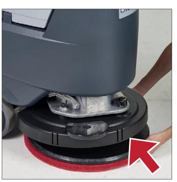
3 Check if the brush are correctly installed and not worn out or if there are external materials avoiding brush rotating.
