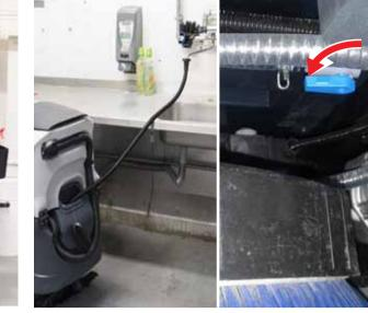
Fill the tank with a clean water. The clean water temperature must not exceed 40 °C.
