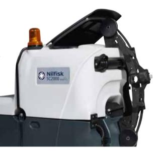
20. Park the machine keeping the recovery tank cover open and hanging the squeegee.
