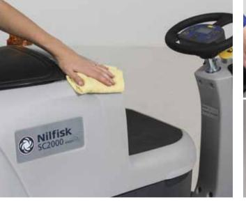
Clean the machine using a damp cloth and where needed use a neutral cleaning product.
