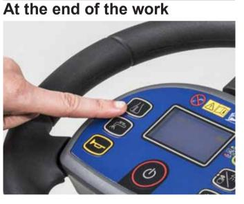
12. Machine with Ecoflex, always end the daily work with turning off the detergent 2 minutes before finishing by pressing the detergent button. To rinse out detergent from the system and brush before handling and cleaning.
