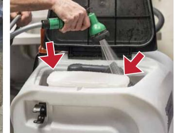
14. Empty the debris tray and clean/ wash the recovery tank inside.
