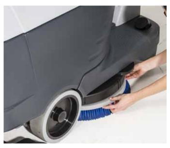
5. Place the brush or the pad-holder under the deck. Use the appropriate brush to clean the floor.
