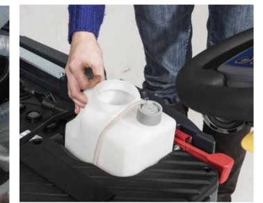
Fill the EcoFlex<sup>™</sup> tank with a detergent suitable for cleaning machines (highly concentrated and low foaming detergent).
