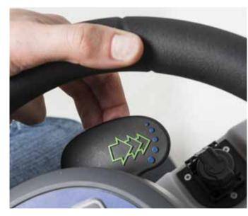
11. Press the EcoFlex<sup>™</sup> lever whenever you temporarily need a greater cleaning power.
