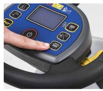
16. Press the click-off button and wait for the brush/pad holder to fall on the floor. Remove to clean or change brush.
